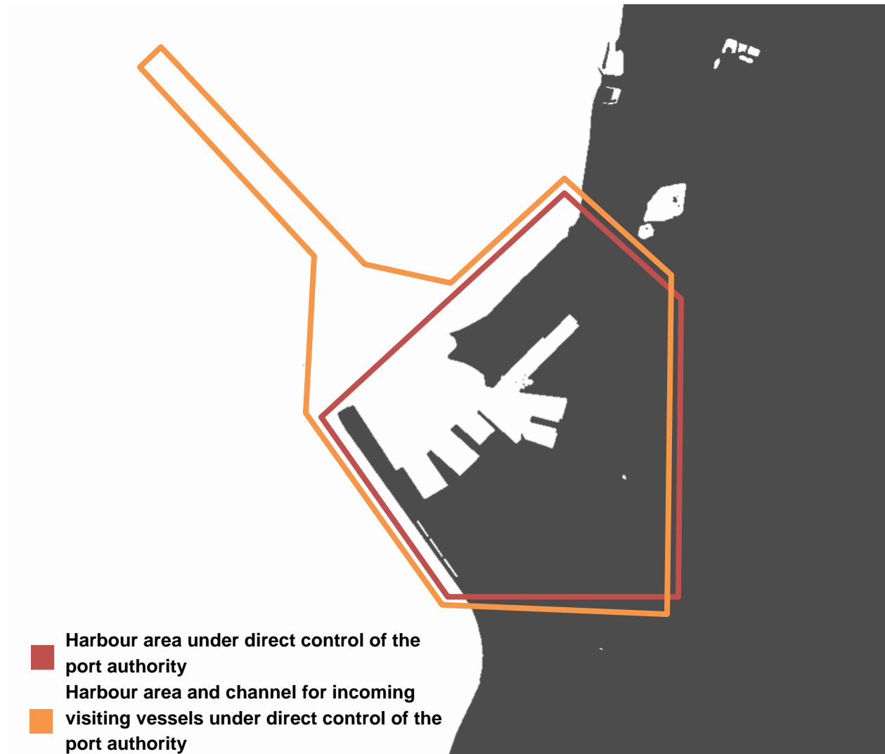
Figure 6. Example for harbour area and channel under control of port authority for the estimation of the manoeuvring time of visiting vessels.
